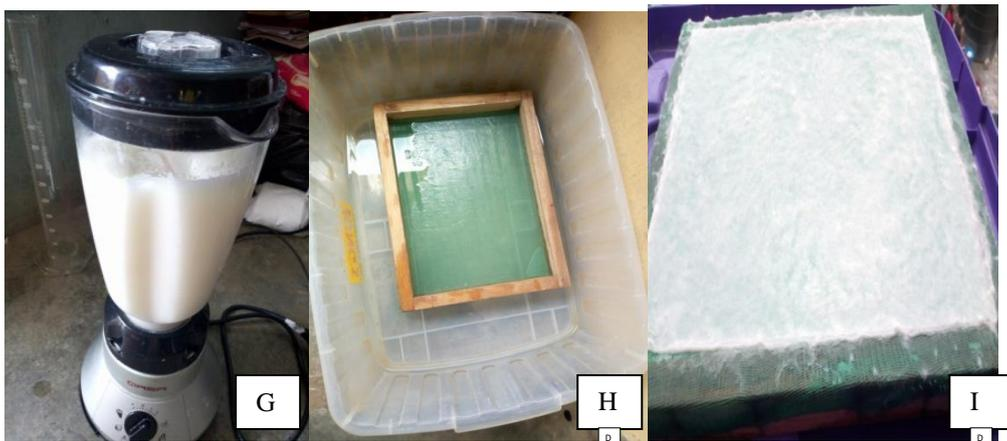
Figure 4: Sheet making process; G = Pulp blending, H = pulp pouring, I = Sheet draining
