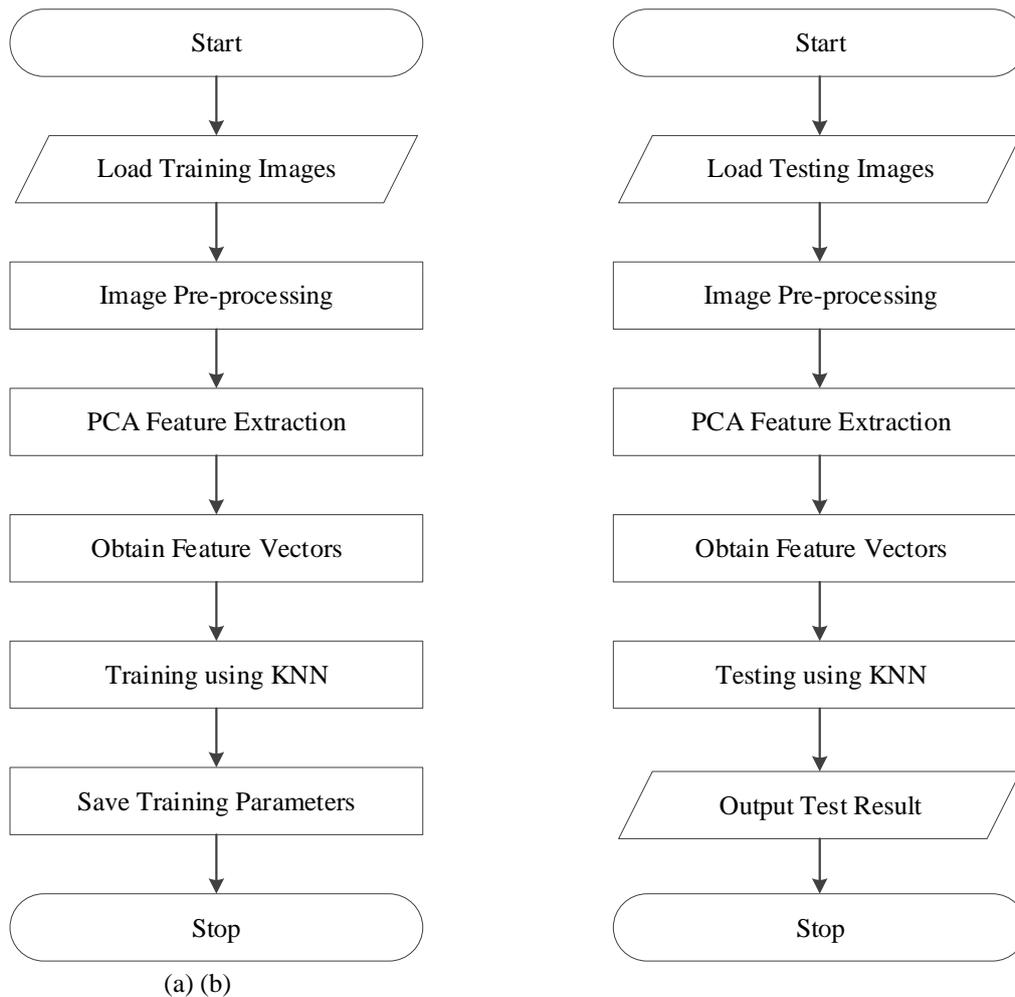
**Figure 2:** Flowchart of the facial recognition (a) training Stage (b) testing Stage
