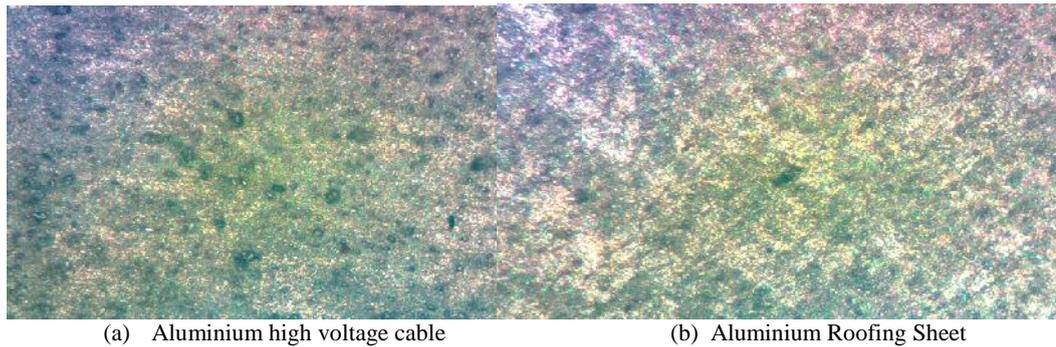
Figure 7: Microstructure of the aluminium high voltage cable and Aluminium Roofing Sheet
