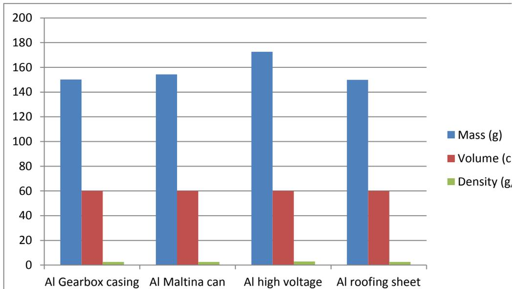
Fig 5: Chart of the mass, volume and density of the aluminium bars
