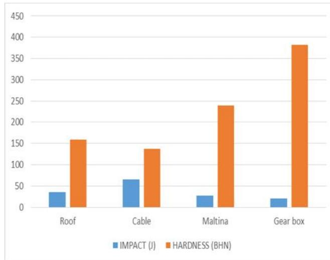
Fig.8: Results of impact and hardness of the materials
