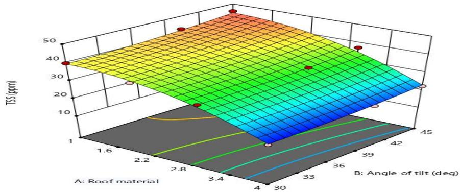
Figure 3: Roof materials and angle of tilt on the TSS
