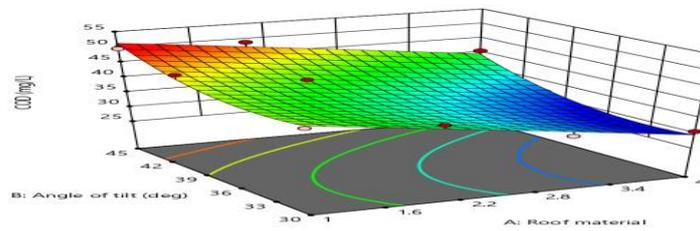
Figure 5: Roof materials and angle of tilt on COD of HR
