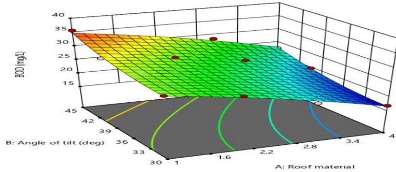
Figure 1: Roof material and angle of tilt on BOD of HR samples
