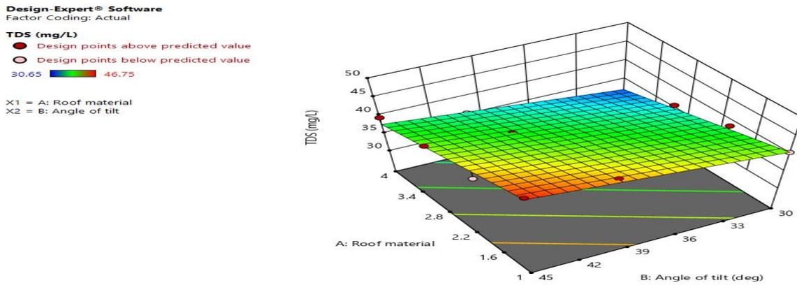
Figure 9: Roof materials and angle of tilt on TDS of HR
