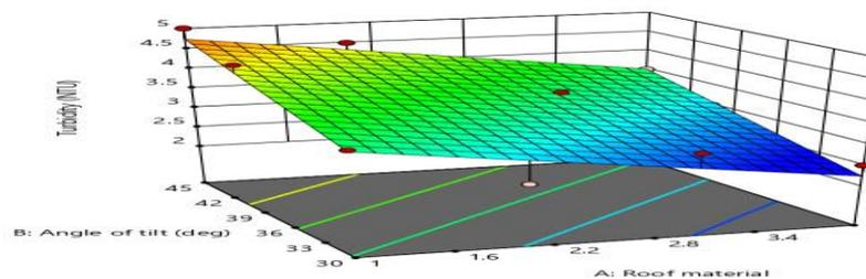
Figure 7: Roof materials and angle of tilt on Turbidity level of HR
