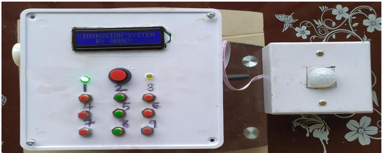
Figure 12: External view of the intrusion detection and alert system
