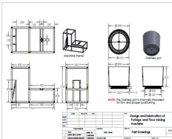
Figure 2: Orthographic Design of the Mixer
