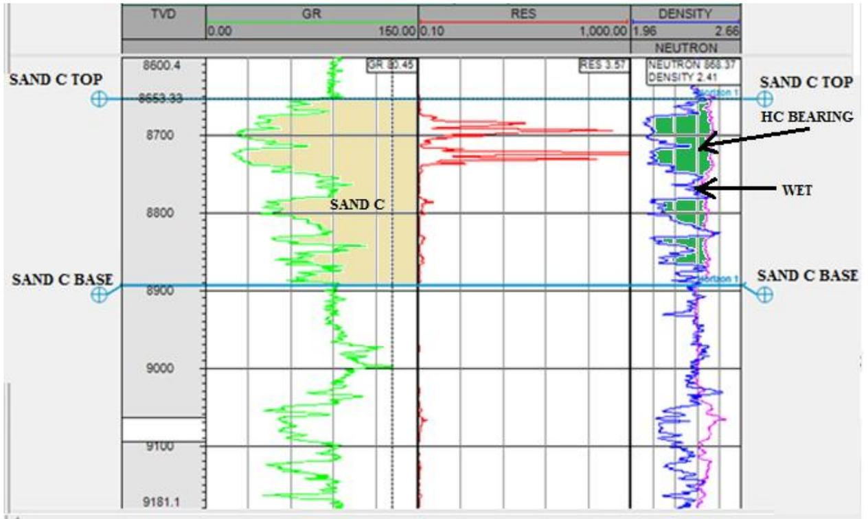
**Fig. 2:** Beta 1 logs showing Reservoir Sand C
