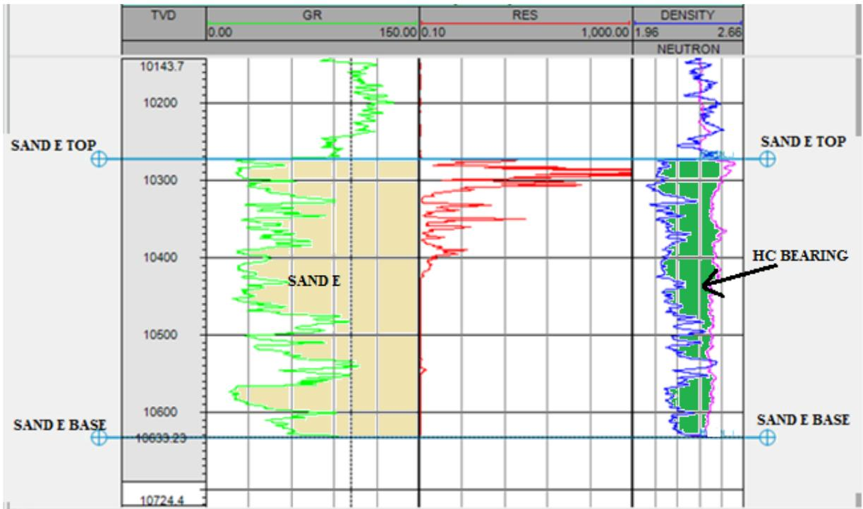
Fig. 3: Beta 3 Logs showing reservoir Sand E
