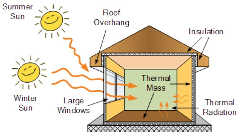
Figure 4: Passive solar energy design considerations (Alternate energy tutorials).
