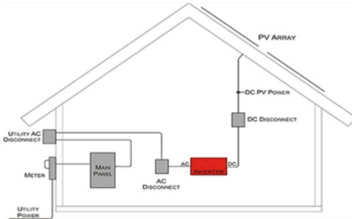
Figure 5: Simple schematic diagram showing PV system incorporated to a home (Robb, 2016).
