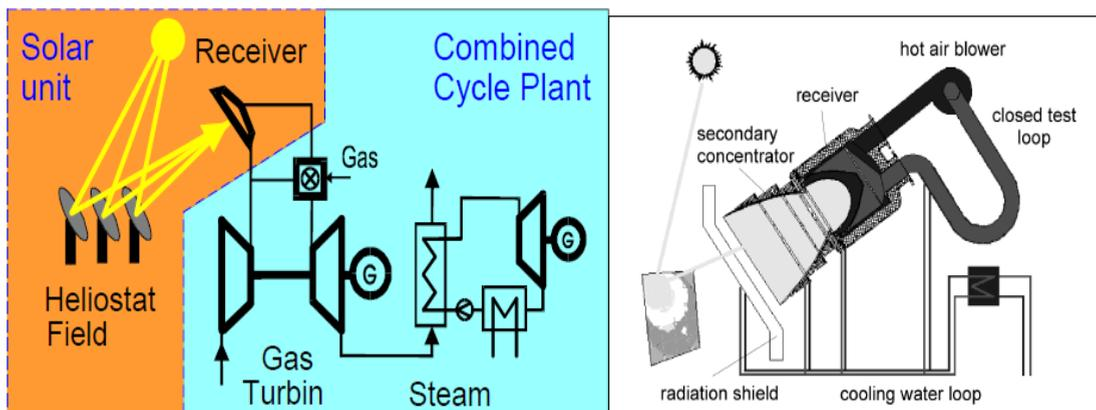
Figure 6: Schematic diagram of solar thermal conversion plant
