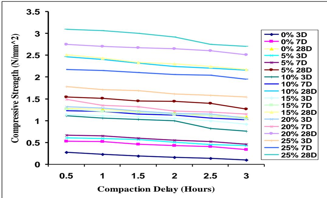
Figure 6: Variation of Compressive Strength of Cement Stabilized Lateritic Blocks with Compaction Delay
