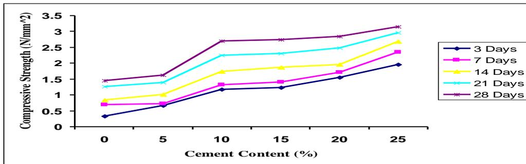
**Figure 5:** Variation of Compressive Strength of Cement Stabilized Lateritic Blocks at no Compaction Delay
