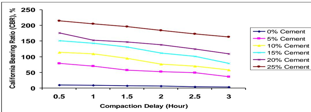
Figure 7: Variation of California Bearing Ratio (CBR) of Cement Stabilized Lateritic Soil with Compaction Delay
