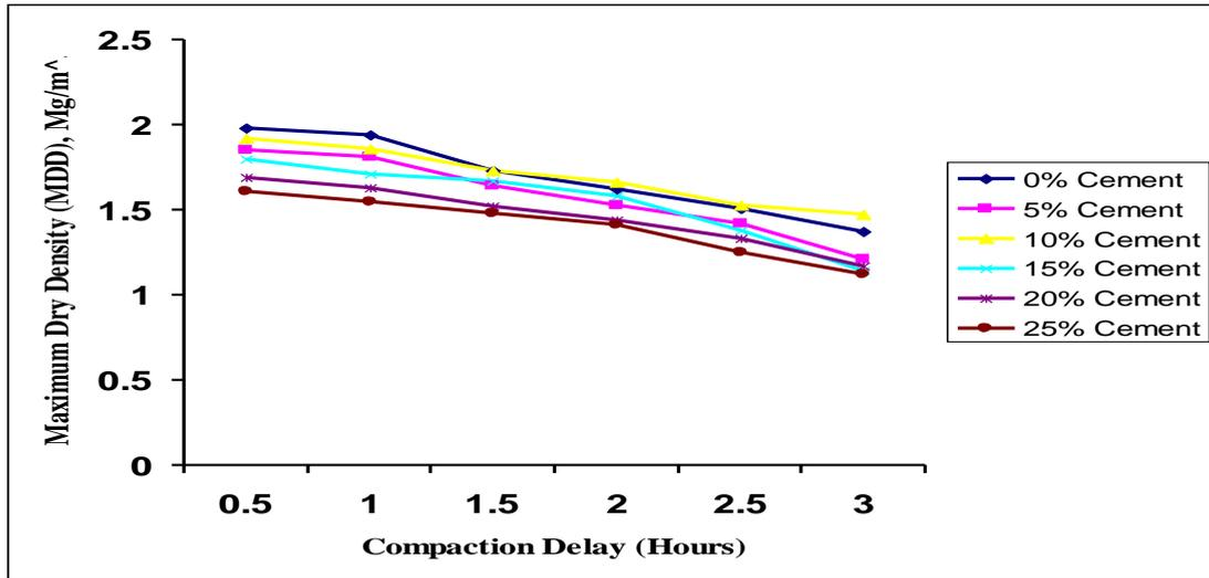
Figure 3: Variation of Maximum Dry Density (MDD) of Stabilized Lateritic Soil with Compaction Delay
