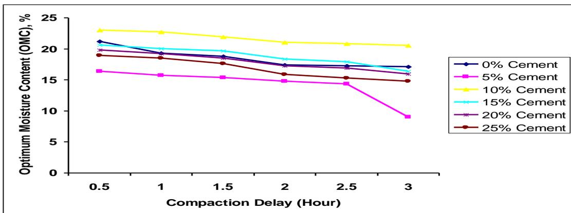
Figure 4: Variation of Optimum Moisture Content (OMC) of Cement Stabilized Lateritic Soil with Compaction Delay
