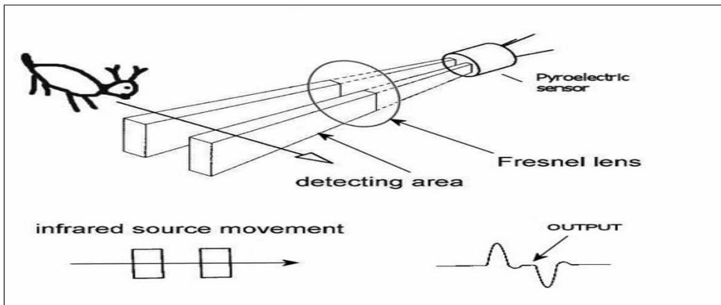
Figure 4: Coverage pattern of the PIR sensor.
