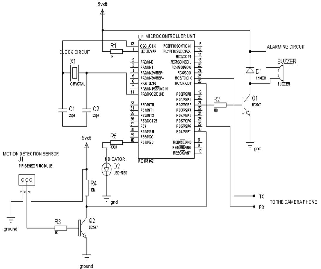
Figure 6: Circuit diagram of the microcontroller connection to PIR sensor.
