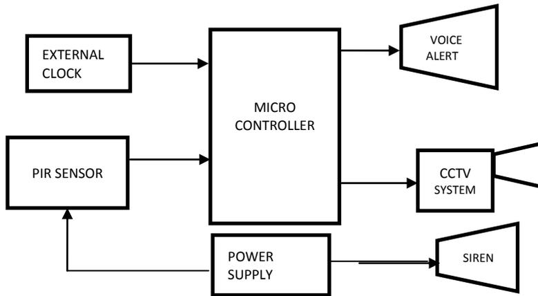
Figure 1: Block diagram of the home security system.
