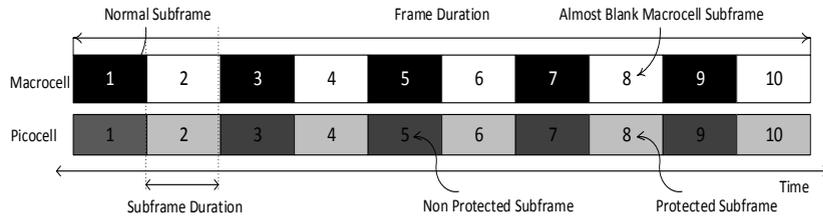
Fig. 2. Use of blank macrocell subframes in 3GPP for interference coordination.
