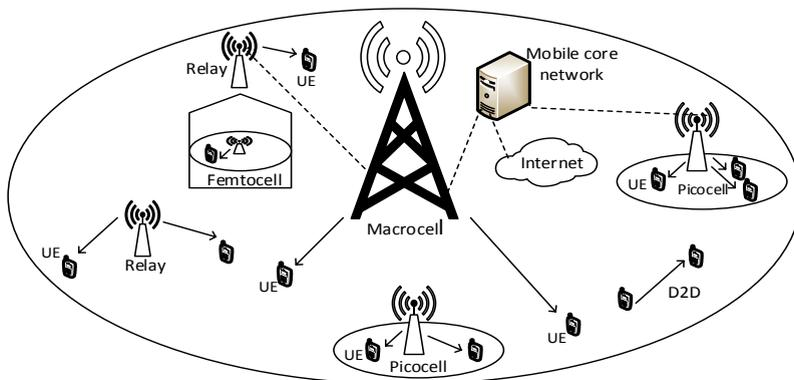
Fig. 1. A multi-tier network composed of macrocells, picocells, femtocells, relays and D2D links. Arrows and dashed lines indicate wireless links and backhaul connections respectively.
