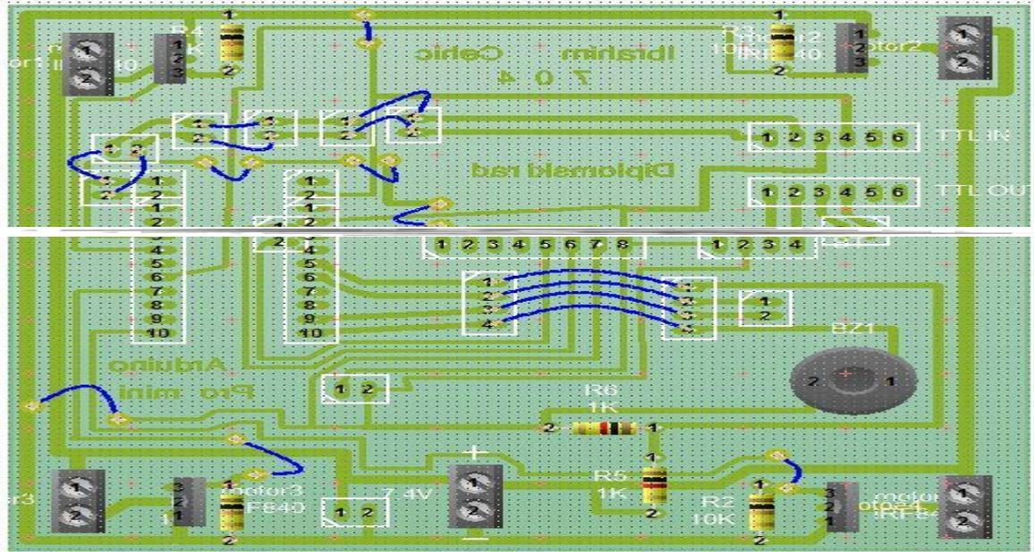
Figure 6: Printed Circuit Diagram of Quadcopter Uncrewed Aerial Vehicle
