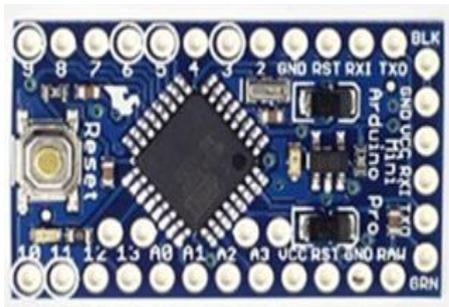
Figure 3: Arduino Pro Mini (ATmega328P)
