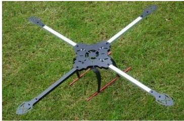
Figure 1: A Quadcopter Frame
