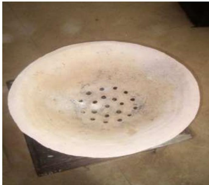
Fig. 2. The perforated ceramic lining of the improved biomass stove.
