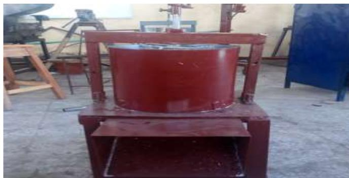
Plate 1: Completed Cassava Shifting Machine
