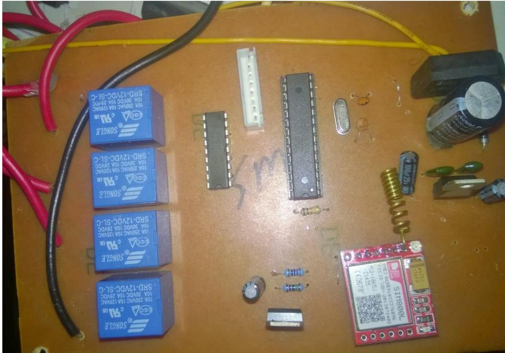
**Fig. 7.** Physical layout of the SMS based device control circuit.
