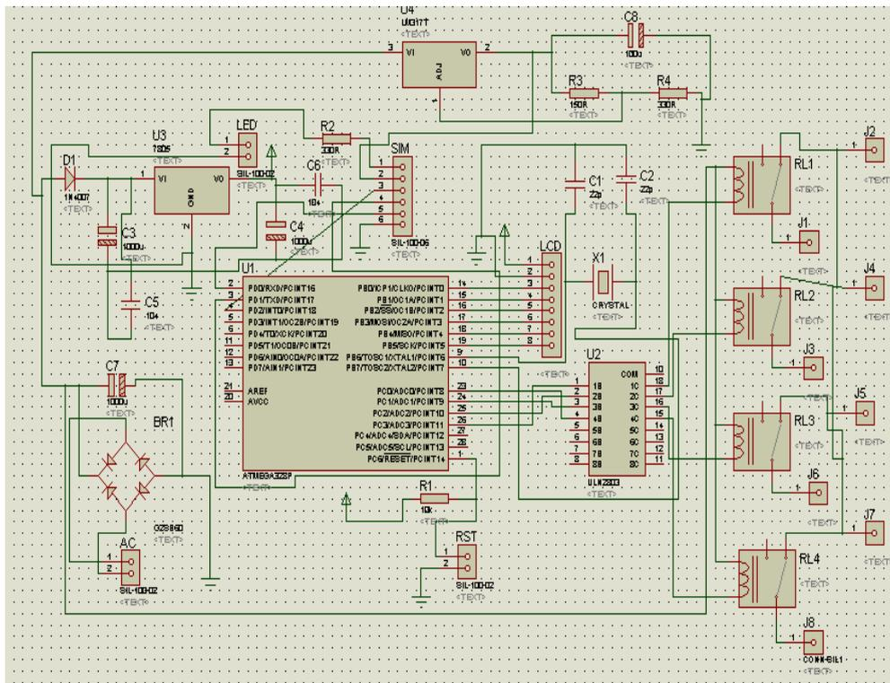
Fig. 6. Circuit diagram of the appliances control.
