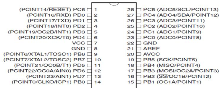
Fig. 3. Pin configuration of ATMEGA 328P Microcontroller.
