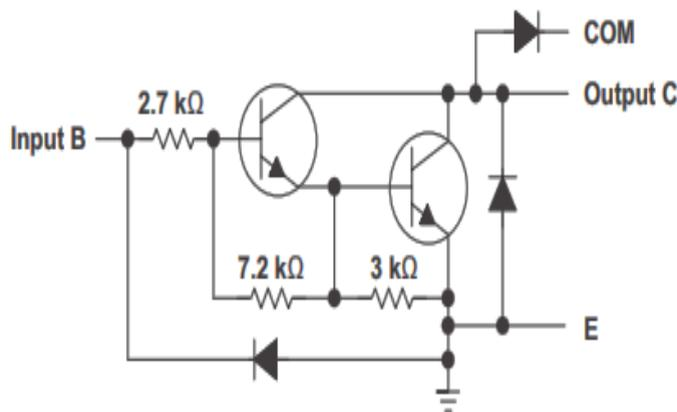
Fig. 5. Internal description of a block of ULN 2803.
