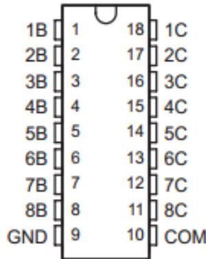
Fig. 4. Pin Configuration of ULN2803
