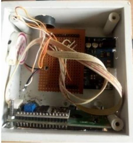
*Figure 3: Internal Packaging of the circuit board*
