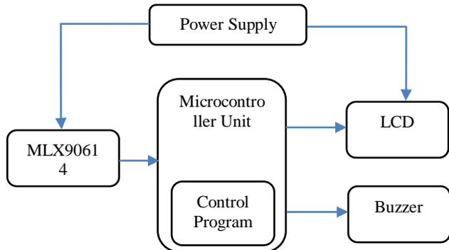
Figure 1: Block diagram of the designed NCFIT
