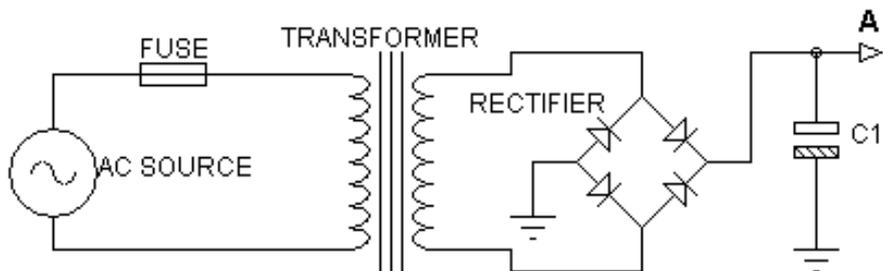
Figure 3: Rectified Power Source for the developed Charger
