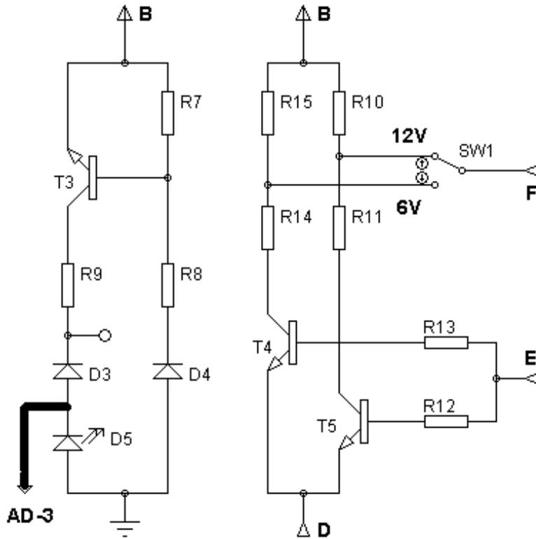
Figure 6: Battery Polarity Monitor and Charging Voltage Selector sections
