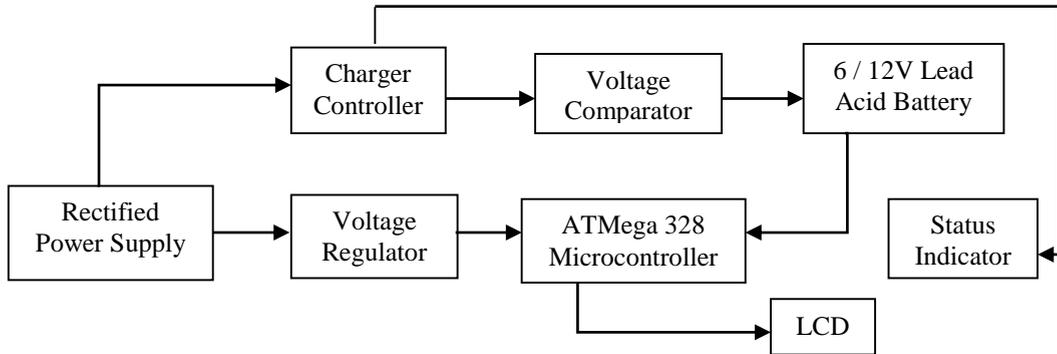
Figure 1: Block Diagram of the Microcontroller based lead acid battery charge
