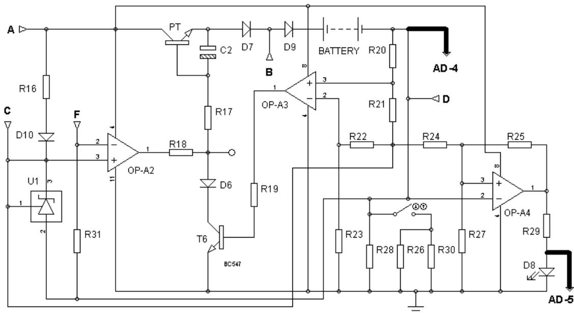
Figure 4: Charging Circuit with Full Charge Status Indicator
