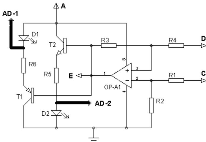
Figure 5: Float Charge and Charging Status Indicator Section
