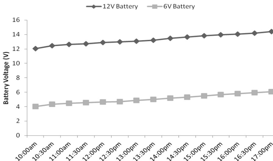
Figure 11: Graphical plot of voltage against time for 12V and 6V battery charging test
