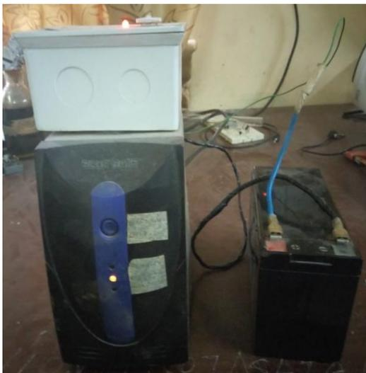
Figure 9: Setup of the developed digital battery charger
