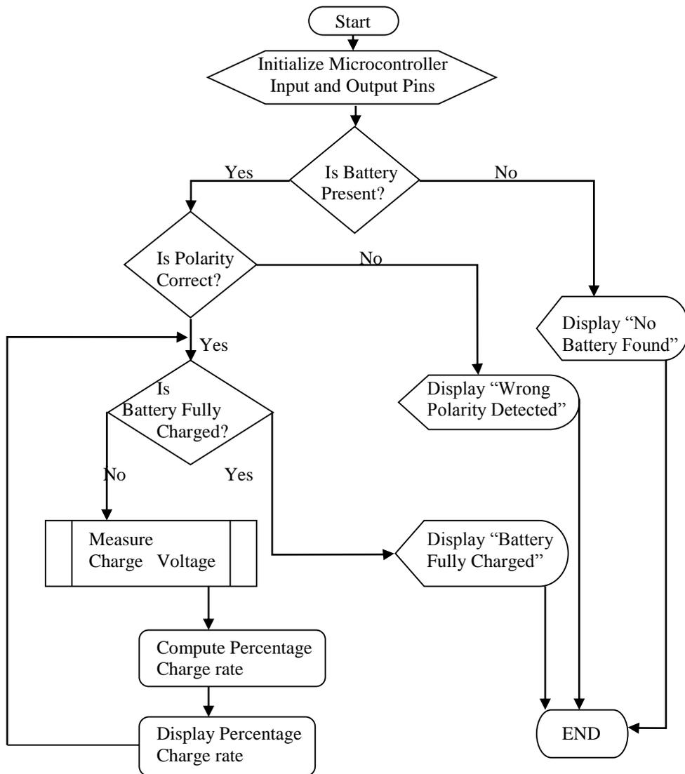
Figure 2: Program Algorithm for the Microcontroller Based Battery Charger
