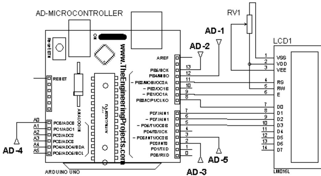
Figure 7: Charger Controller Section with LCD connections
