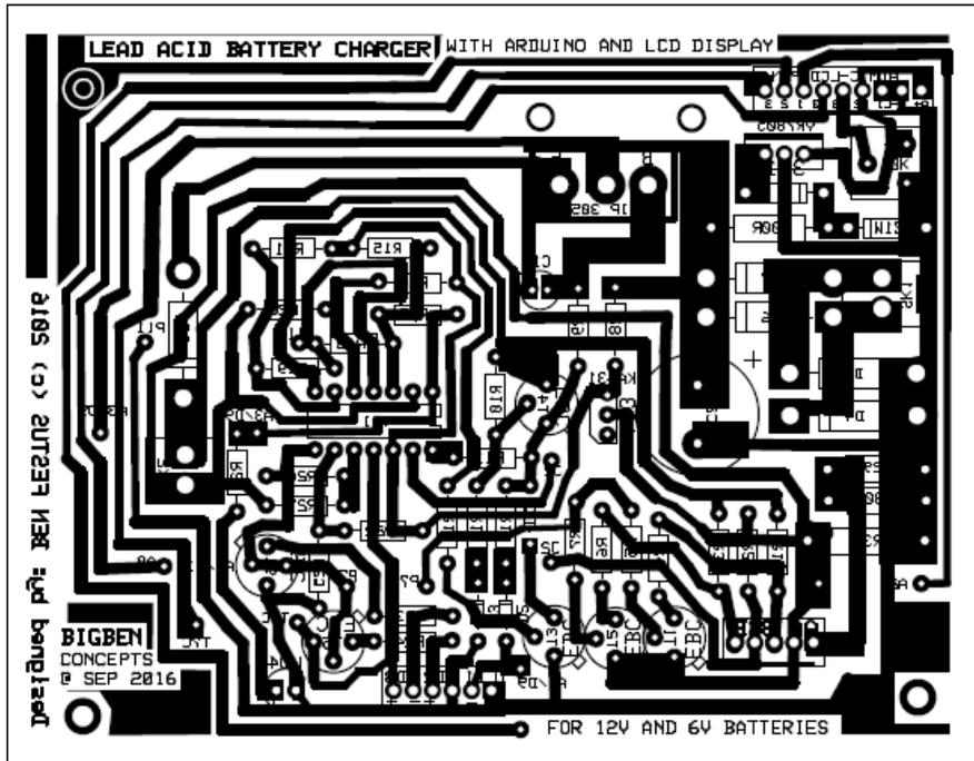
Figure 8: PCB developed for the improved battery charger project
