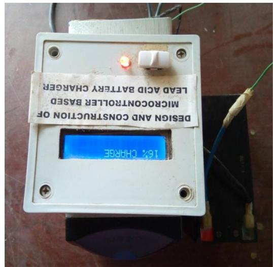
Figure 10: Cross-section of the Digital Battery charger showing charging rate
