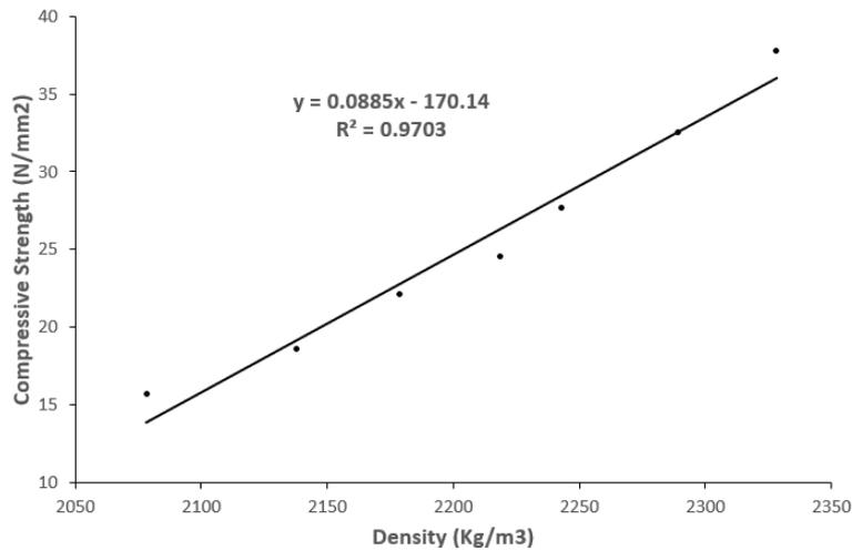
Figure 3: Relationship between density and compressive strength for W/C Ratio of 0.40
