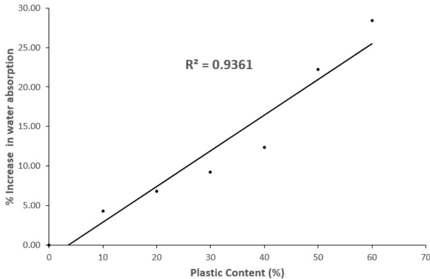
Figure 2: Relationship between plastic content and % increase in water absorption
