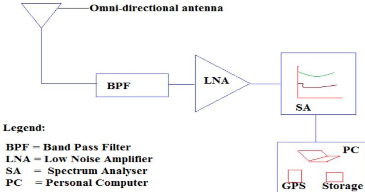
**Figure 3: The diagrammatic measurement Set-up**
