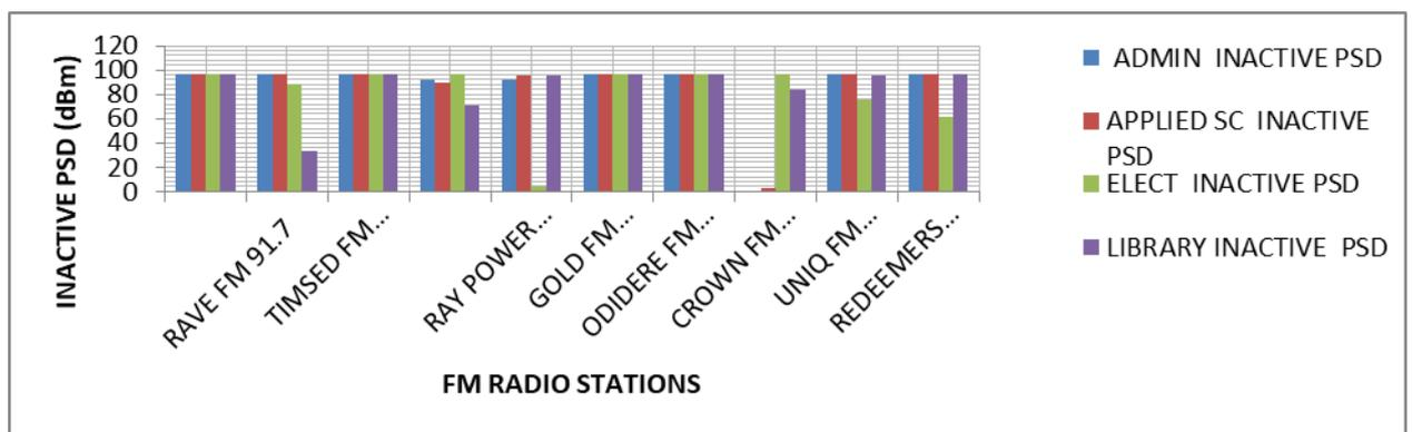
Figure 5: FM Stations Inactive Power Spectral Density Distribution within 8 hours period.
