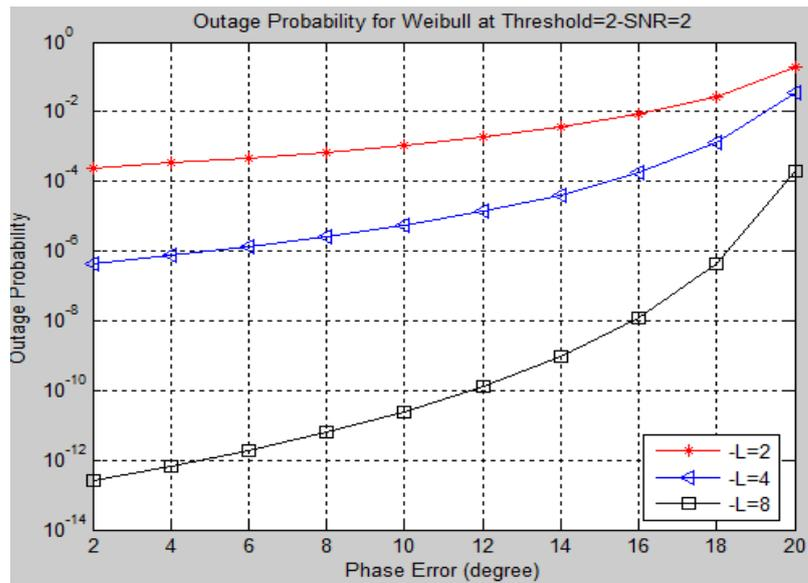
Figure 3: Theoretical Outage Probability versus Phase Error at SNR of 2 dB and a threshold value of 2 dB over Weibull fading channel at L of 2, 4 and 8
