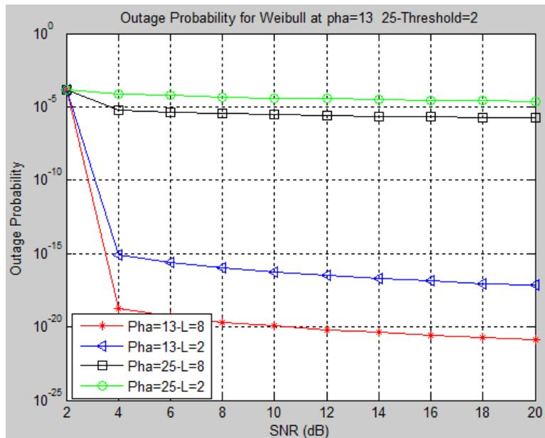
Figure 6: Theoretical Outage Probability versus SNR at a PE (pha) of  $13^\circ$  and  $25^\circ$  with threshold value of 2 dB over Weibull fading channel at L of 2 and 8
