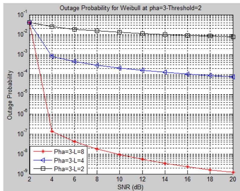
Figure 4: Theoretical Outage Probability versus SNR at a PE (pha) of  $3^\circ$  and a threshold value of 2 dB over Weibull fading channel at L of 2, 4 and 8
