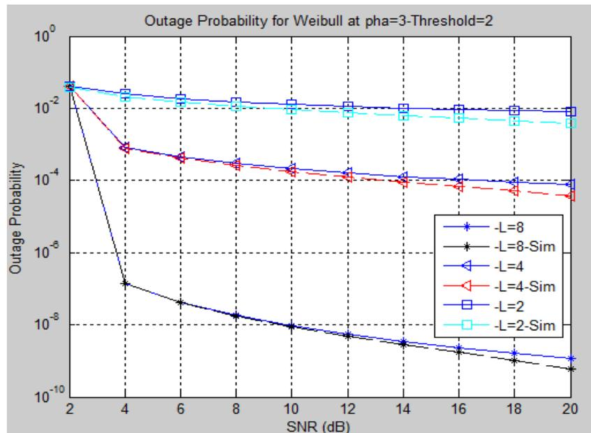
Figure 7: Simulation and Theoretical Outage Probability versus SNR at a PE (pha) of  $3^\circ$  and a threshold value of 2 dB over Weibull fading channel at L of 2, 4 and 8
