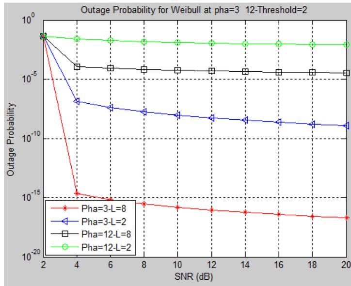
Figure 5: Theoretical Outage Probability versus SNR at a PE (pha) of  $3^\circ$  and  $12^\circ$  with threshold value of 2 dB over Weibull fading channel at L of 2 and 8
