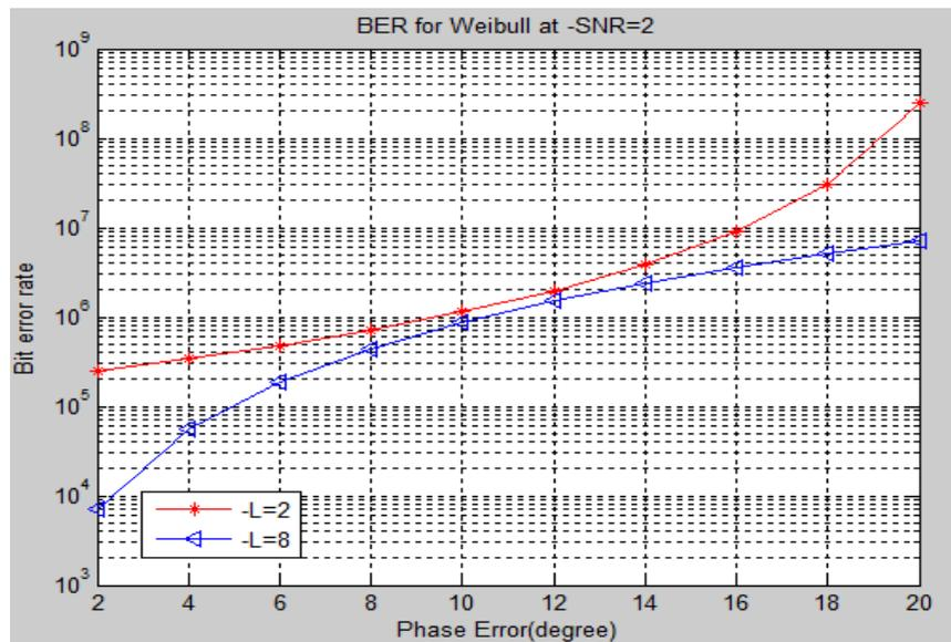
Figure 2: Theoretical Bit Error Rate of BPSK modulated signal versus Phase Error at SNR of 2 dB over Weibull fading channel at L of 2 and 8
