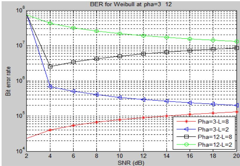
Figure 1: Theoretical Bit Error Rate of BPSK modulated signal versus SNR at PE of 3° and 12° over Weibull fading channel at L of 2 and 8
