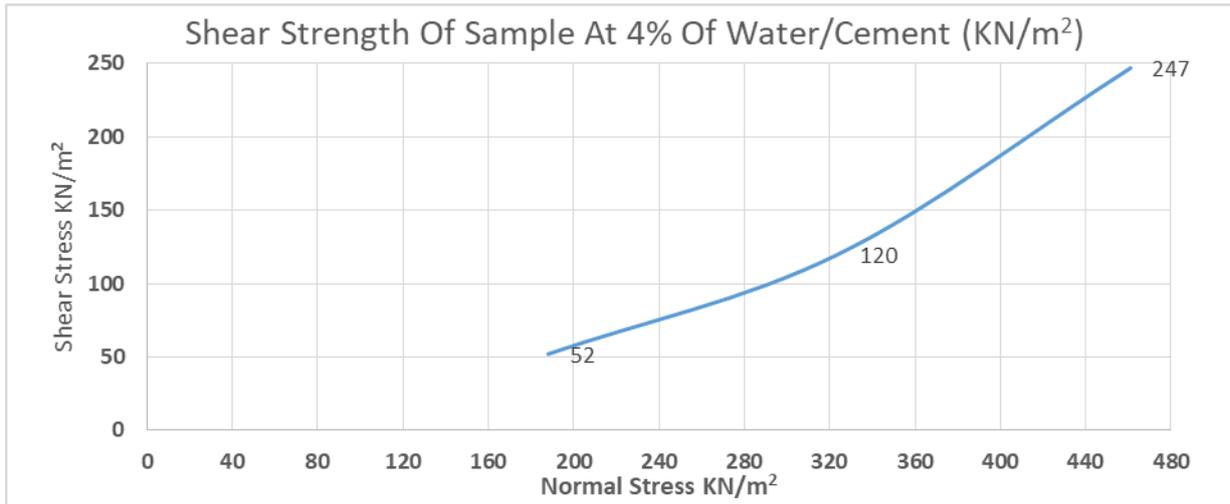
Figure 3: Shear Stress - Normal Stress (KN/m<sup>2</sup>) at 4% Water/Cement
