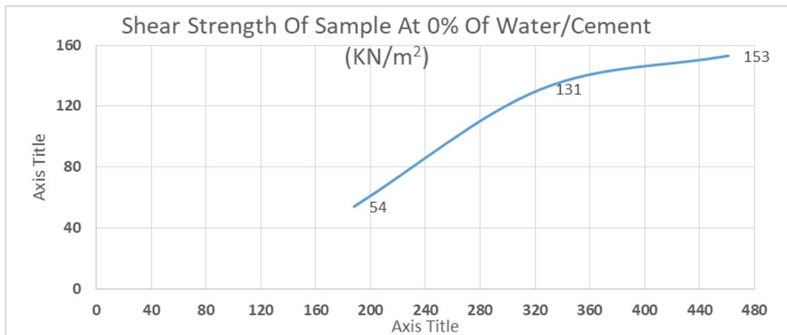
Figure 1: Shear Stress - Normal Stress (KN/m<sup>2</sup>) at 0% Water/Cement
