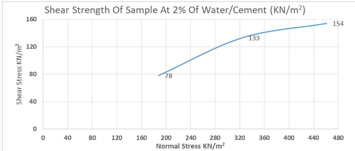
Figure 2: Shear Stress - Normal Stress (KN/m<sup>2</sup>) at 2% Water/Cement
