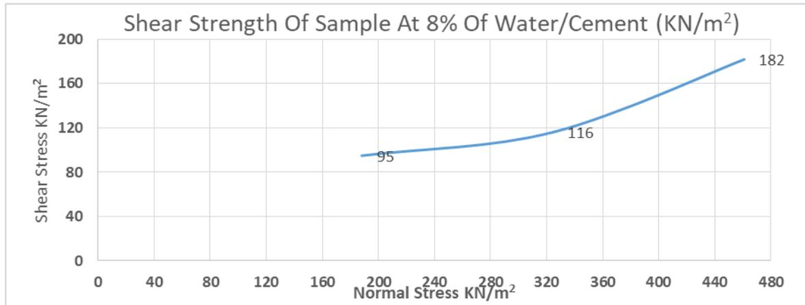
Figure 5: Shear Stress - Normal Stress (KN/m<sup>2</sup>) at 8% Water/Cement
