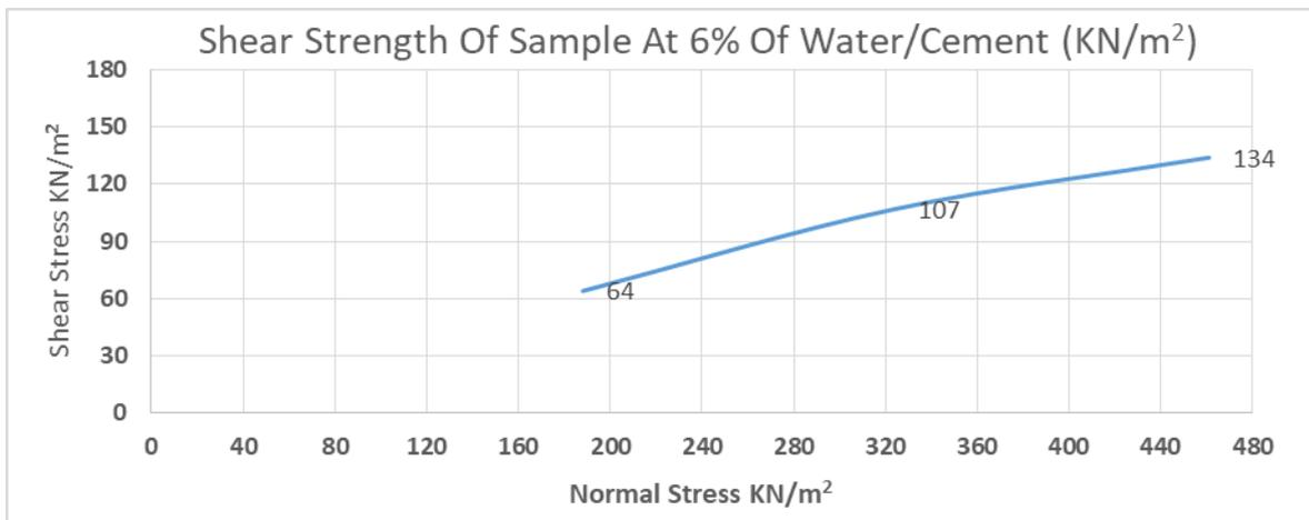
Figure 4: Shear Stress - Normal Stress (KN/m<sup>2</sup>) at 6% Water/Cement
