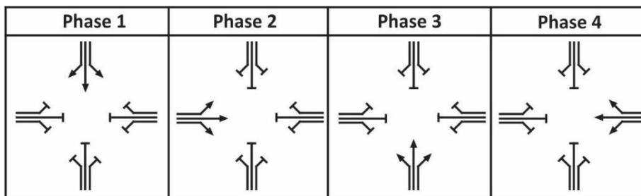
Fig.2 Existing phase design of Ibara signalized intersection
