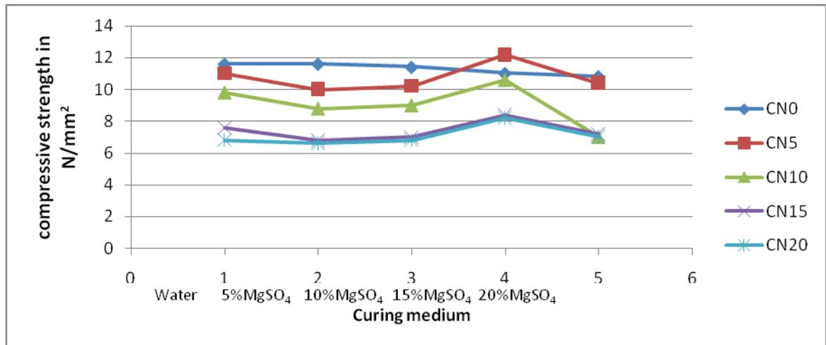
**Figure 7:** Compressive strength of OPC and OPC/SCBA cured in water and 0%,5%,10%,15%,20% Solution of MgSO<sub>4</sub> at 14 days of hydration
