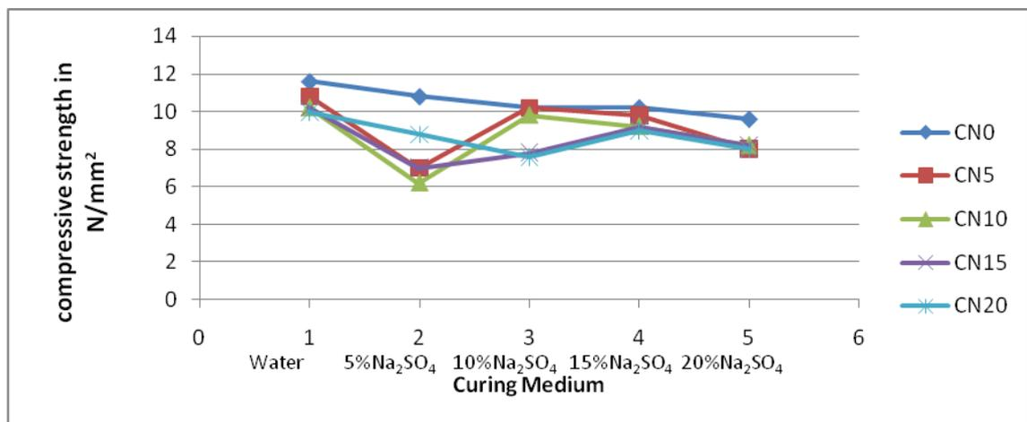
**Figure 4:** Compressive strength of OPC and OPC/SCBA cured in water and 0%,5%,10%,15%,20% and solution of Na<sub>2</sub>SO<sub>4</sub> at 14days of hydration
