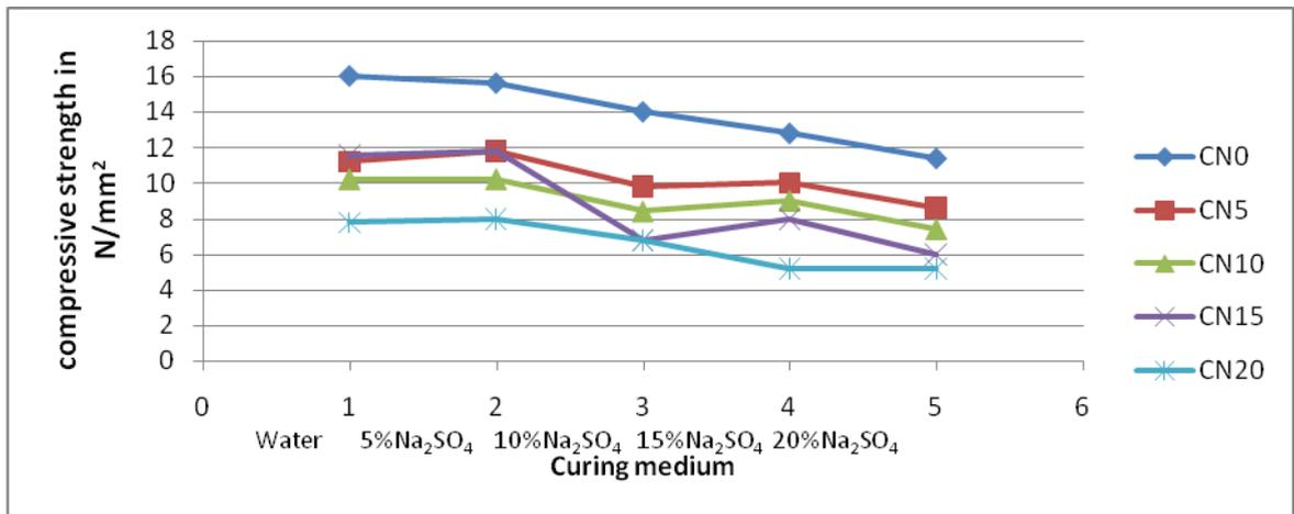
**Figure 6:** Compressive strength of OPC and OPC/SCBC cured in water and solution Na<sub>2</sub>SO<sub>4</sub> in 28 days of hydration.
