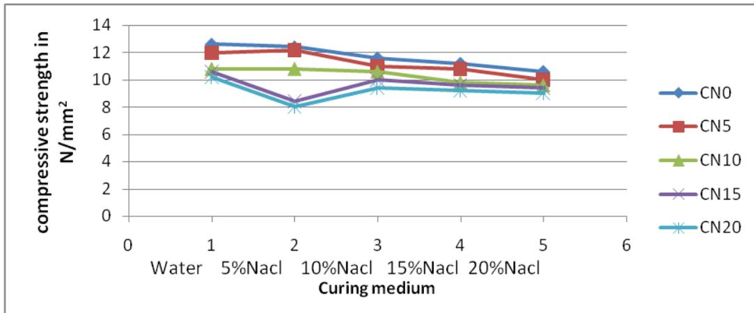
**Figure 2:** Compressive Strength of OPC and OPC/SCBA cured in water and 5%,10%,15%,20% solution of NaCl at 21days of hydration.
