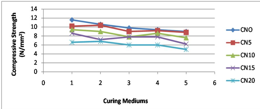
**Figure 1:** Compressive Strength of OPC and OPC/SCBA cured in water and 5%,10%,15%,20% solution of NaCl<sub>2</sub> at 14days of hydration.
