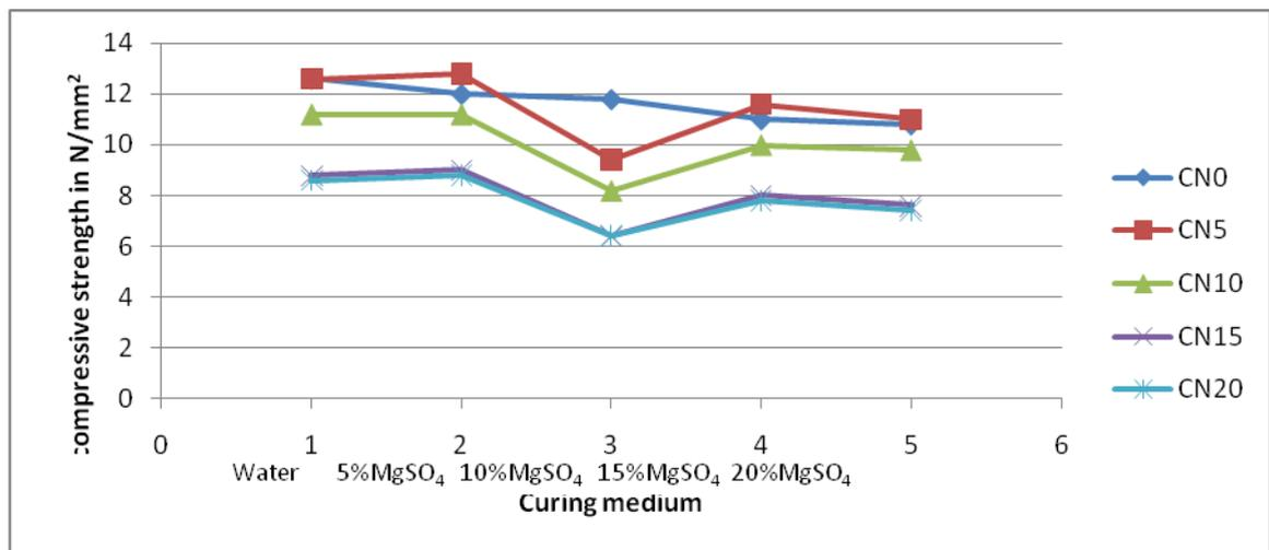
**Figure 8:** Compressive strength of OPC and OPC/SCBA cured in water and 0%,5%,10%,15%,20% Solution of MgSO<sub>4</sub> at 21 days of hydration.
