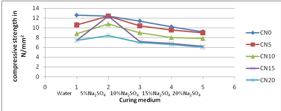
**Figure 5:** Compressive strength of OPC and OPC/SCBA cured in water and 0%,5%,10%,15%,20% Solution of Na<sub>2</sub>SO<sub>4</sub> at 21 days of hydration.
