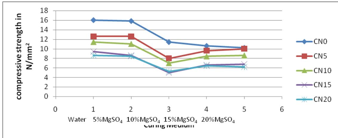
**Figure 9:** Compressive strength of OPC and OPC/SCBA cured in water and 0%,5%,10%,15%,20% Solution of MgSO<sub>4</sub> at 28 days of hydration
