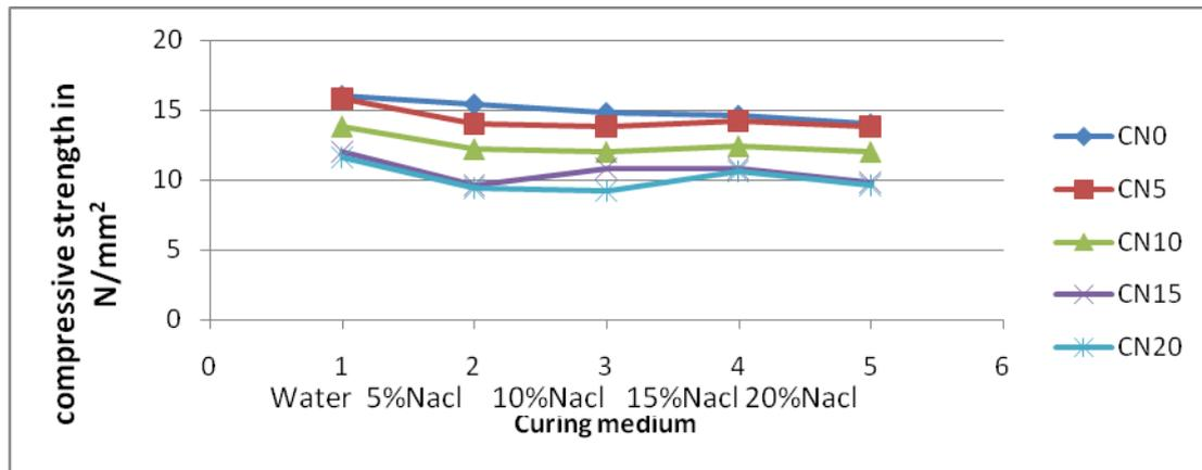
**Figure 3:** Compressive strength of OPC and OPC/SCBA cured in water and 0%,5%,10%,15%,20% solution of NaCl<sub>2</sub> at 28days of hydration.
