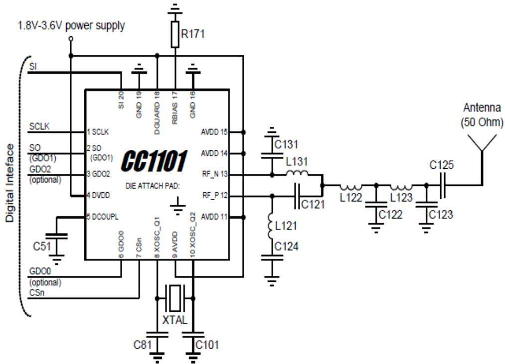
Figure 1: CC1101 circuit diagram
