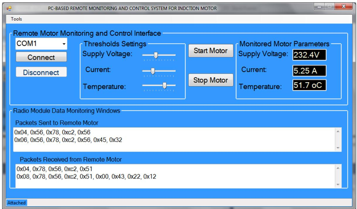
Figure 7: Motor monitoring and control interface
