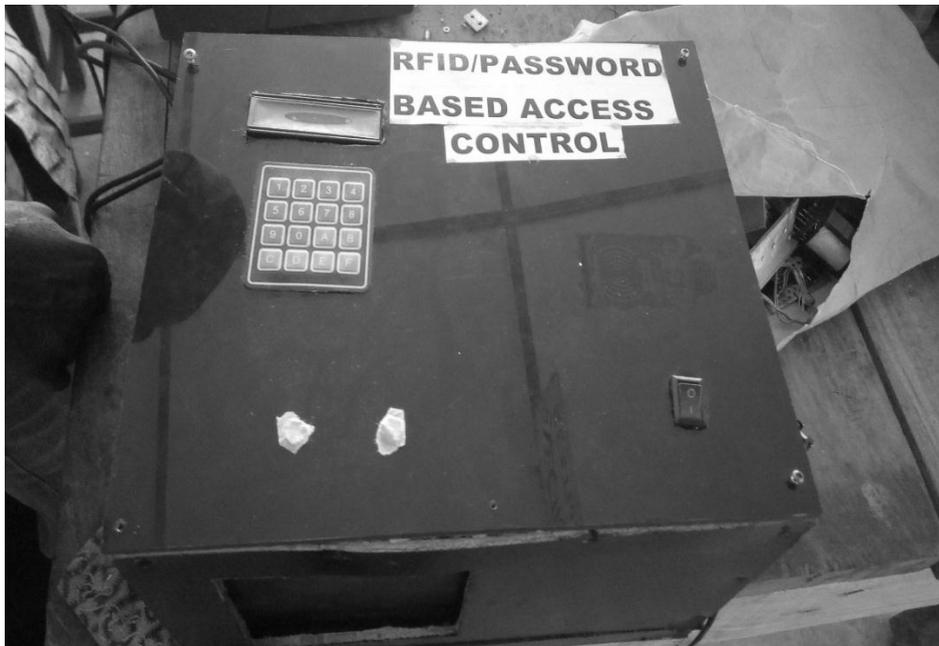
**Figure 4:** Complete prototype RFID/Password based door access control system.
