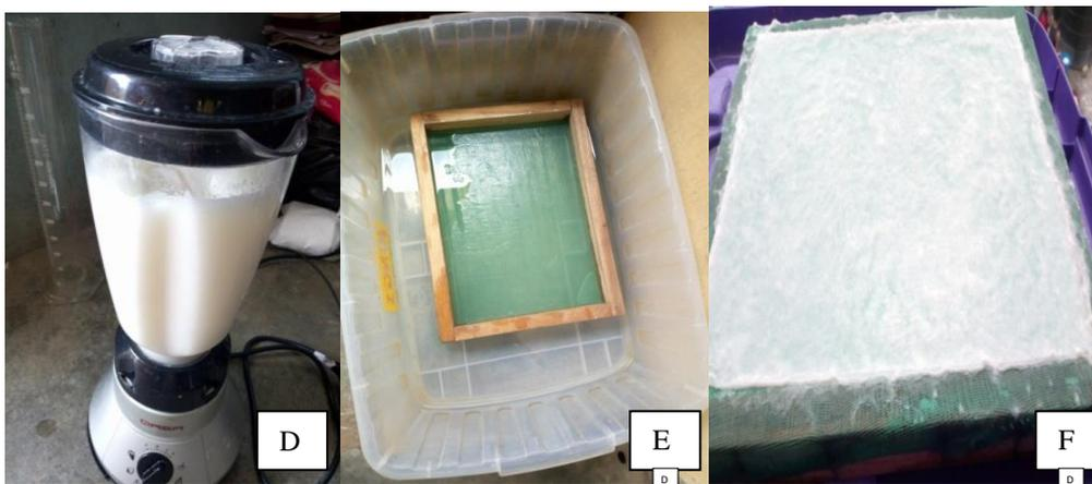
Figure 4: Sheet making process; D = Pulp blending, E = pulp pouring, F = Sheet draining
