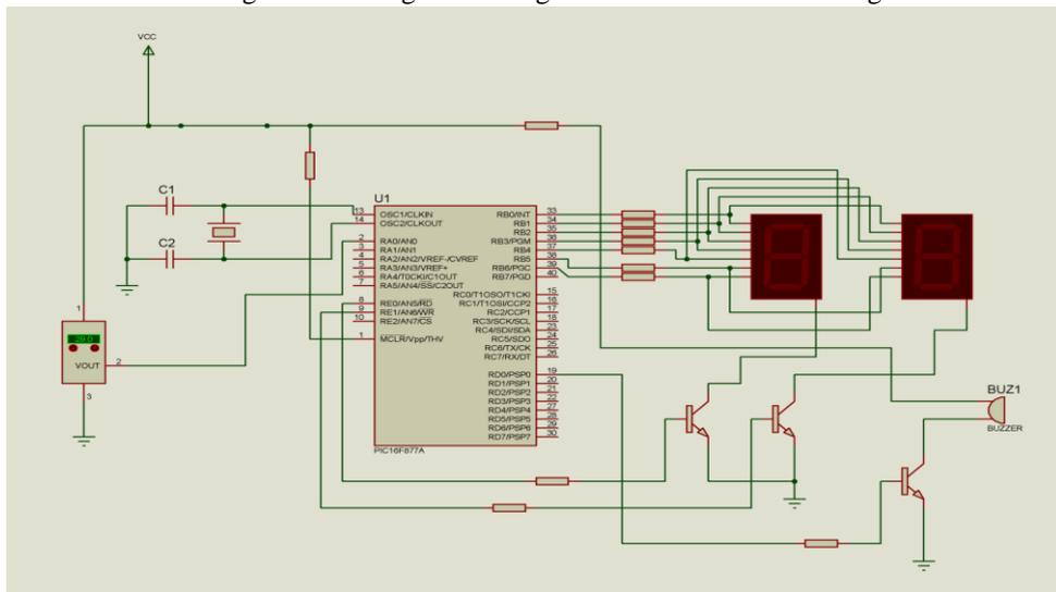
Fig. 2. Digital thermometer circuit diagram
