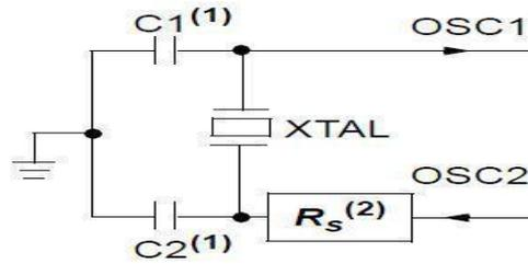
Fig. 4. Crystal oscillator set-up diagram [6]
