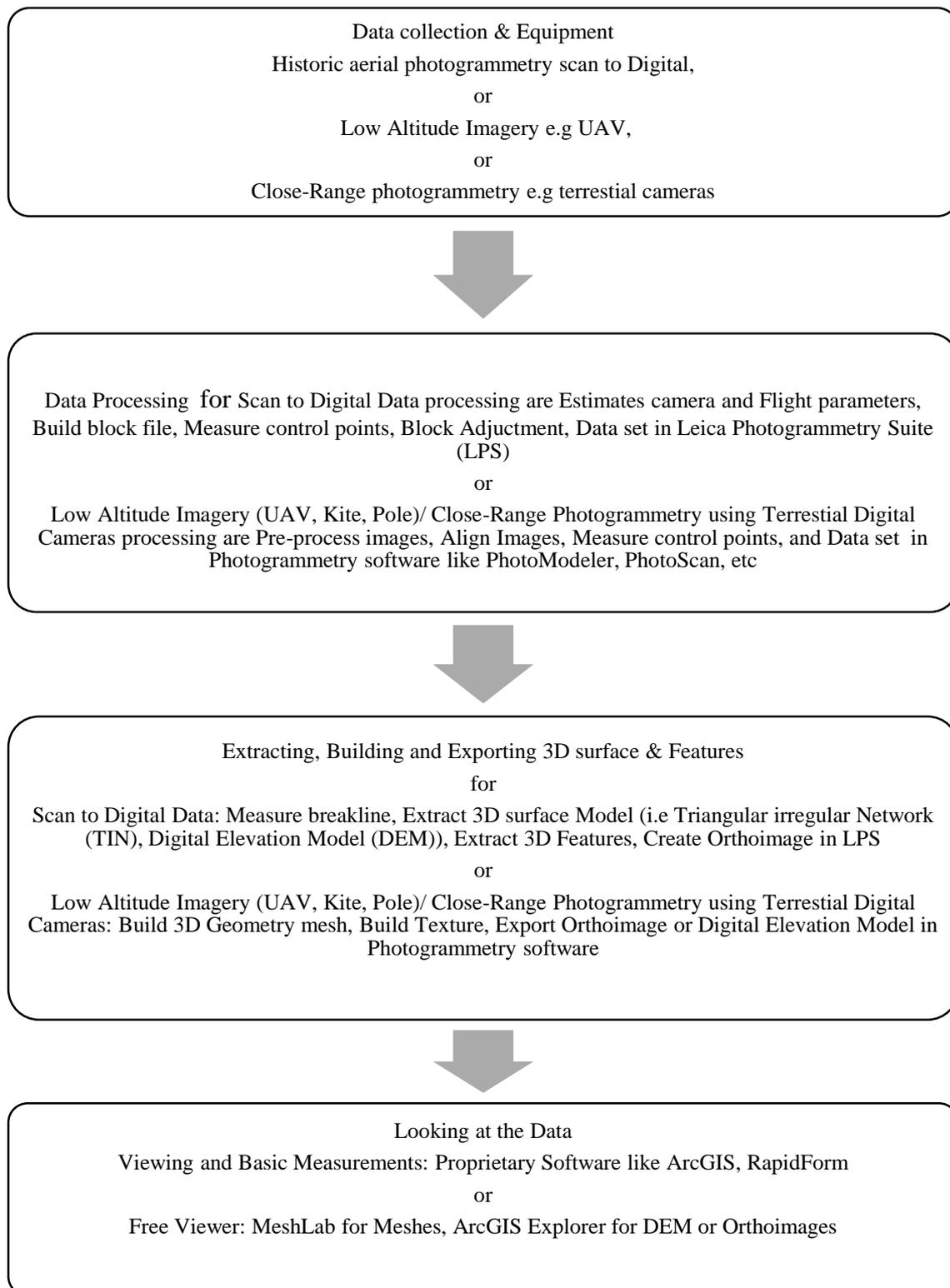
Figure 1.1 Basic Digital Photogrammetry workflow
