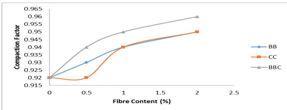
Figure 2: Compaction Factor – Fibre Content Characteristics for the Concrete Cubes
