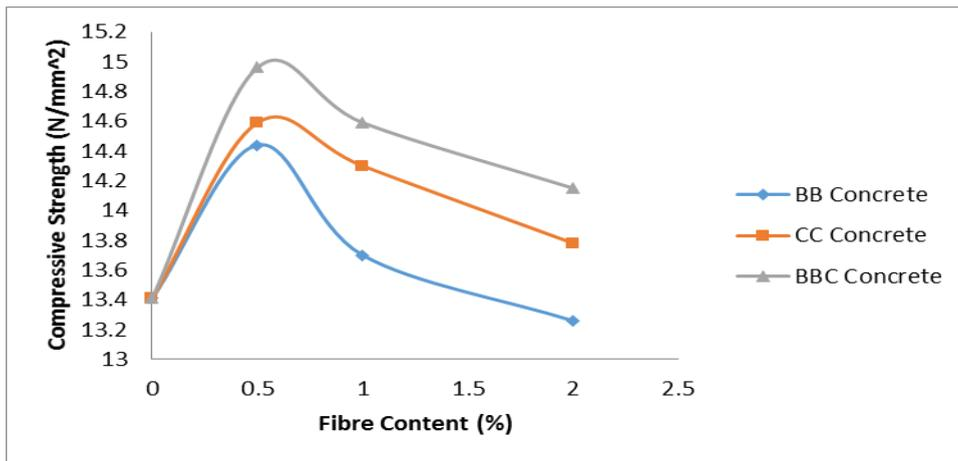
Figure 3: Compressive Strength – Fibre Content Characteristics for the Concrete Cubes
