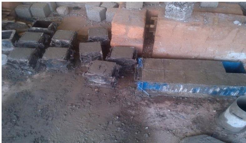
**Plate 1: Concrete cubes placed in moulds**
