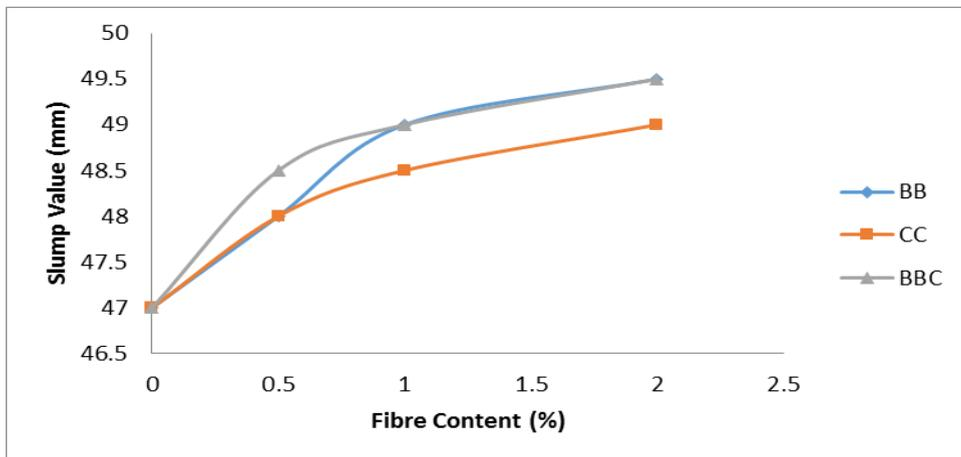
Figure 1: Slump Value – Fibre Content Characteristics for the Concrete Cubes
