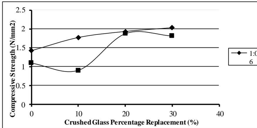
Figure 1: Graph showing strength of sandcrete hollow block with mix 1:6 and 1:8 cured with water for 7 days
