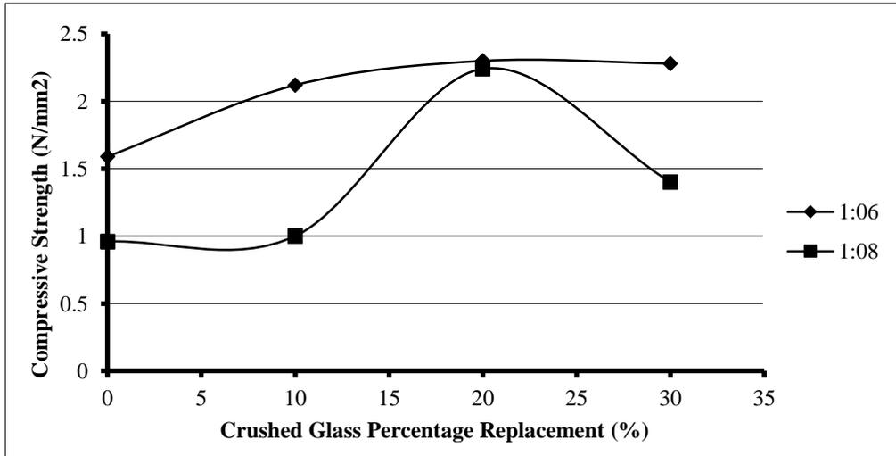
Figure 3: Graph showing strength of sandcrete hollow block with mix 1:6 and 1:8 cured with MgSO<sub>4</sub> at 7 days
