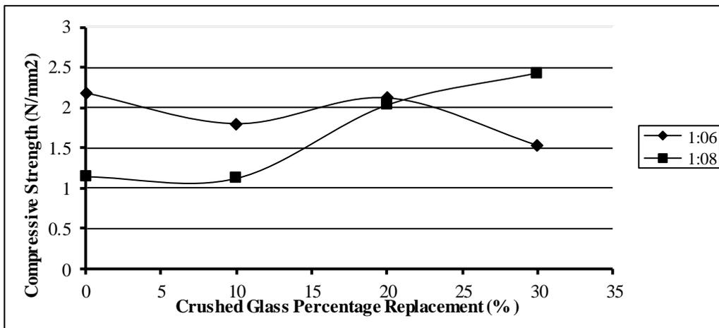
Figure 2: Graph showing strength of sandcrete hollow block with mix 1:6 and 1:8 cured with water for 14 days
