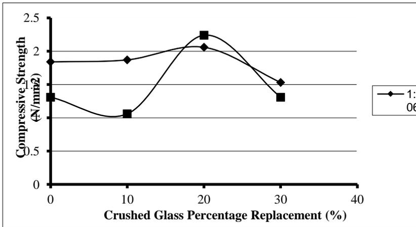
Figure 4: Graph showing strength of sandcrete hollow block with mix 1:6 and 1:8 cured with MgSO<sub>4</sub> at 14 days
