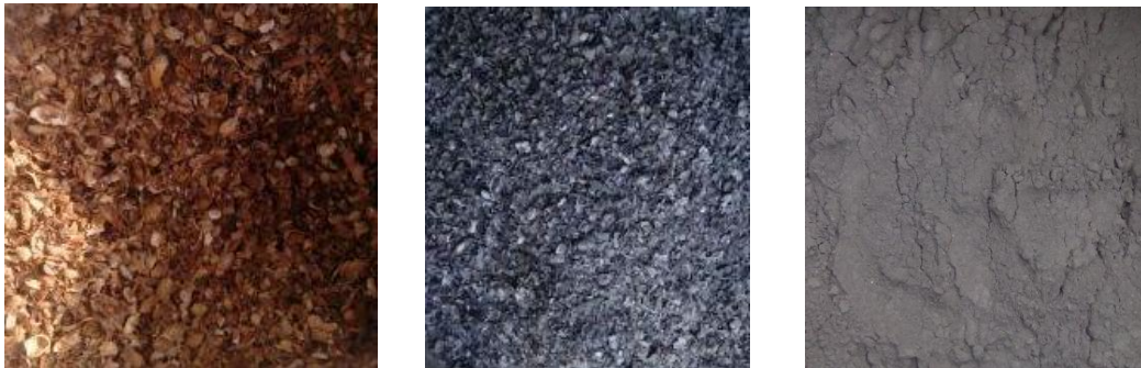
Fig. 1. (a) Groundnut Shell, (b) Groundnut Shell Ash and (c) Grinded Groundnut Shell Ash
